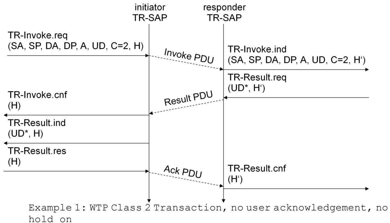
The initiator can indicate the successful transmission of the invoke message and the result with the two service primitives **TR-Invoke.cnf** and **TR-Result.ind**. A user may respond to this result with **TR-Result.res**. An acknowledgement PDU is then generated which finally triggers the **TR-Result.cnf** primitive on the responder's side. This example clearly shows the combination of
