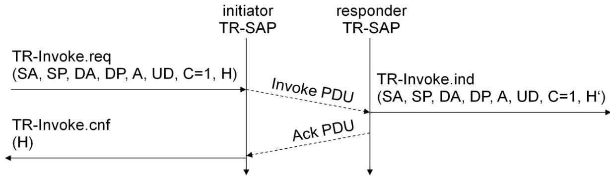
The responder signals the incoming invoke PDU via the **TR-Invoke.ind** primitive to the higher layer and acknowledges automatically without user intervention. For the initiator the transaction ends with the reception of the acknowledgement. The responder keeps the transaction state for some time to be able to retransmit the acknowledgement if it receives the same invoke PDU again indicating a loss of the acknowledgement.
