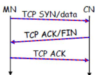
T/TCP can combine packets for connection establishment and connection release with user data packets. This can reduce the number of packets down to two instead of seven. The obvious **advantage** for certain applications is the reduction in the overhead which standard TCP has for connection setup and connection release. Disadvantage is that it requires changes in the software in mobile host
