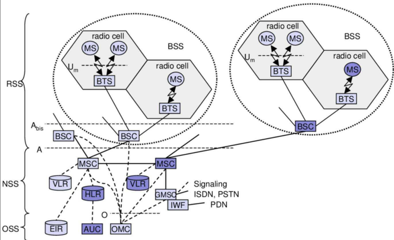
Functional Architecture of a GSM System
