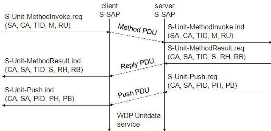
The function of the **S-Unit-MethodResult** primitive remains the same as explained above: the **status (S)**, **response header (RH)**, and **response body (RB)** represent the result of the operation. The **S-Unit-Push** primitive has the parameters **client address (CA)**, **server address (SA)**, **push identifier (PID)**, **push header (PH)**, and **push body (PB)**.
