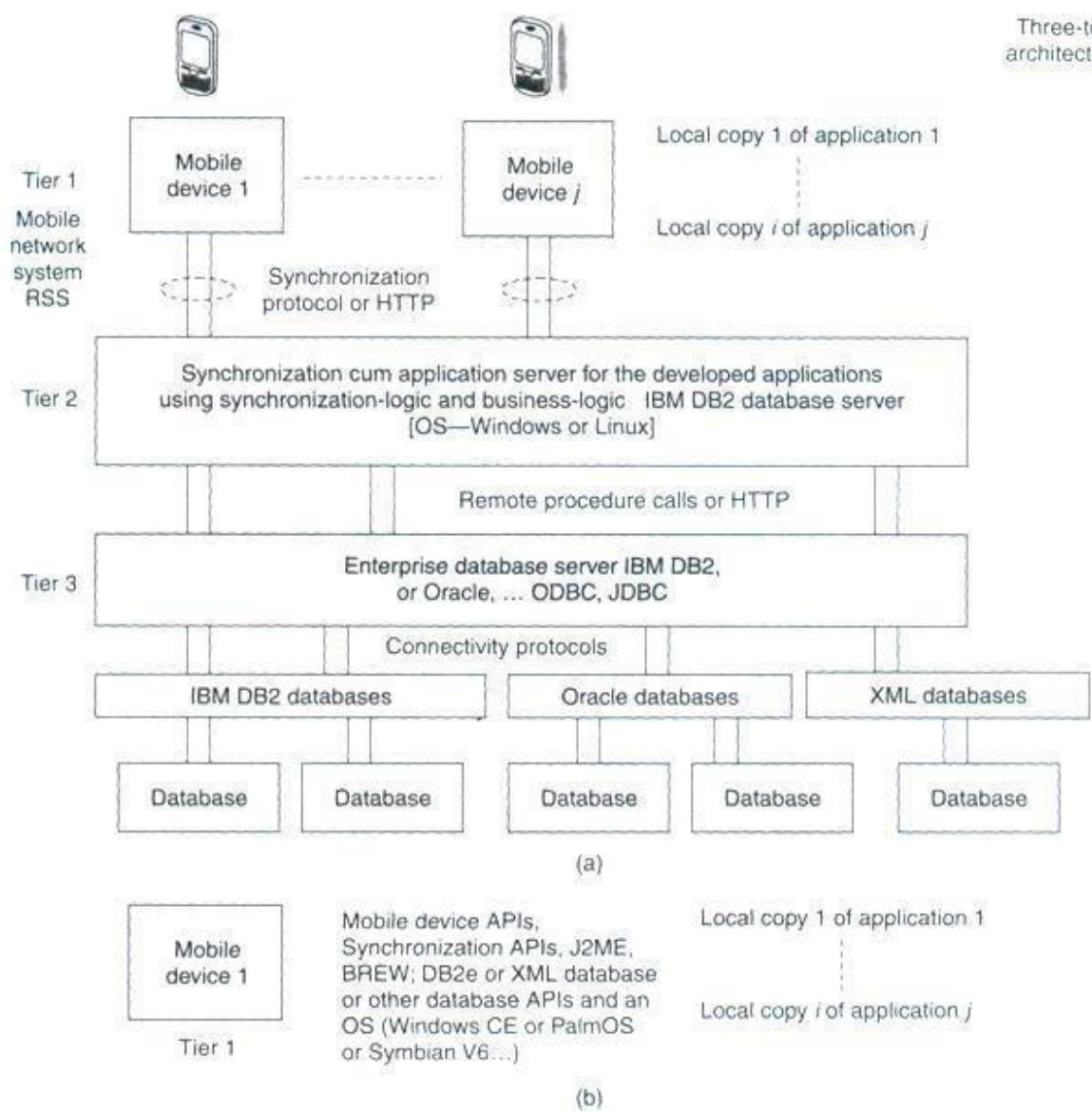
**(a) Local copies 1 to  $j$  of database hoarded at the mobile devices using an enterprise database connectionsynchronizationserver, which synchronizes the required local copies for application with the enterprise database server (b) Mobile device with J2ME or BREW platform, APIs an OS and database having localcopies**
