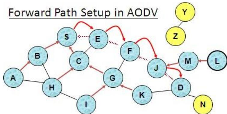
Forward links are setup when RREP travels along the reverse path
