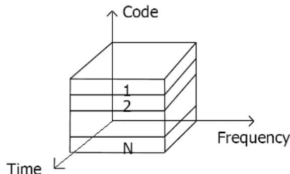
All terminals send on the same frequency probably at the same time and can use the whole bandwidth of the transmission channel. Each sender has a unique random number, the sender XORs the signal with this random number. The receiver can “tune” into this signal if it knows the pseudo random number, tuning is done via a correlation function
