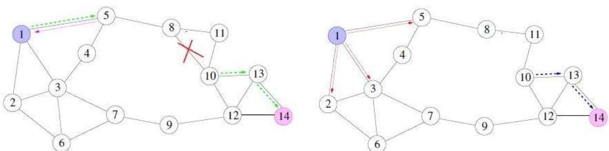
A routing table entry maintaining a reverse path is purged after a timeout interval. Timeout should be long enough to allow RREP to come back. A routing table entry maintaining a forward path is purged if *not used* for a *active\_route\_timeout* interval. If no data is being sent using a particular routing table entry, that entry will be deleted from the routing table (even if the route may actually still be valid).
