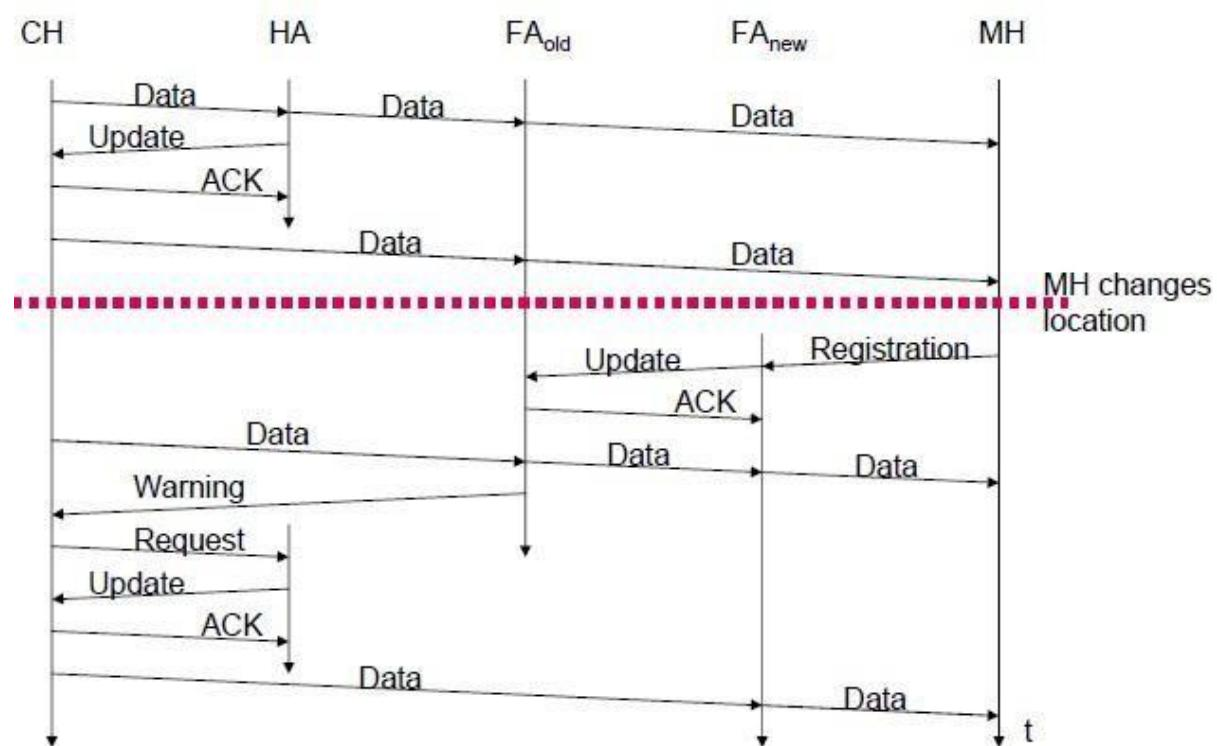
The CN can request the current location from the HA. If allowed by the MN, the HA returns the COA of the MN via an update message. The CN acknowledges this update message and stores the mobility binding. Now the CN can send its data directly to the current foreign agent FA<sub>old</sub>. FA<sub>old</sub> forwards the packets to the MN. This scenario shows a COA located at an FA. Encapsulation of data for tunneling to the COA is now done by the CN, not the HA.
