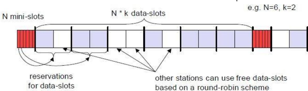
This guarantees each station a certain bandwidth and a fixed delay. Other stations can now send data in unused data-slots as shown. Using these free slots can be based on a simple round-robin scheme or can be uncoordinated using an Aloha scheme. This scheme allows for the combination of, e.g., isochronous traffic with fixed bitrates and best-effort traffic without any guarantees.
