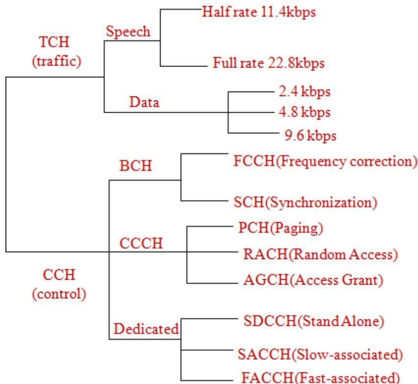
**Control Channels:** Control channels carry system signalling and synchronisation data for control procedures such as location registration, mobile station synchronisation, paging, random access etc. between base station and mobile station. Three categories of control channel are defined: Broadcast, Common and Dedicated. Control channels are multiplexed into the 51-frame multiframe.
