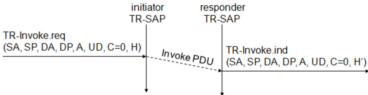
Additionally, with the **A** flag, the user of this service can determine, if the responder WTP entity should generate an **acknowledgement** or if a user acknowledgement should be used. The WTP layer will transmit the **user data (UD)** transparently to its destination. The class type **C** indicates here class 0. Finally, the transaction **handle H** provides a simple index to uniquely
