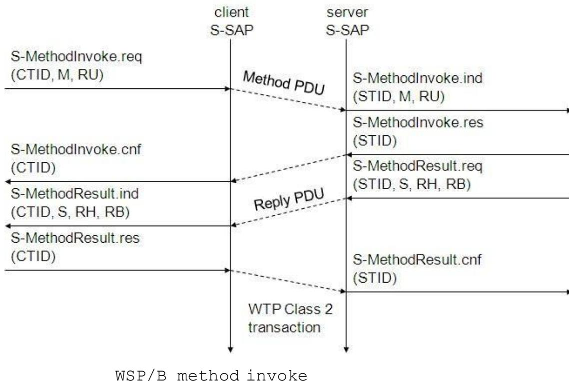
A client requests an operation with **S-MethodInvoke.req**. Parameters are the **client transaction identifier CTID** to distinguish between pending transactions, the **method M** identifying the requested operation at the server, and the **request URI** (Uniform Resource Identifier **RU**). The WTP class 2 transaction service now transports the **method PDU** to the server. A method PDU can be either a get PDU or a post PDU.
