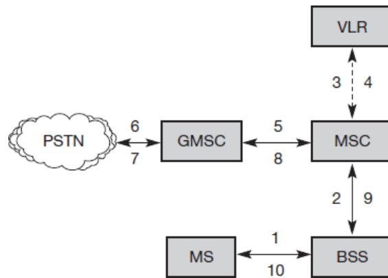
**step 1:** The MS transmits a request for a new connection
