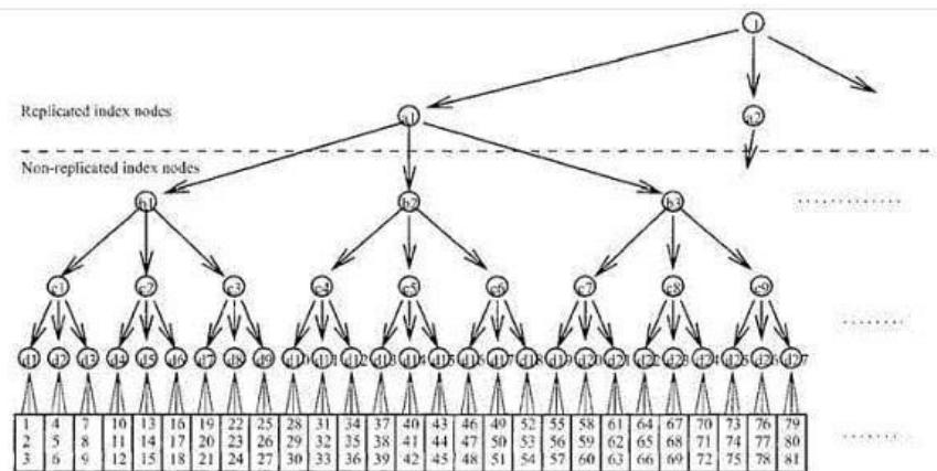
Figure 4.4. A partial data file and its index tree.
