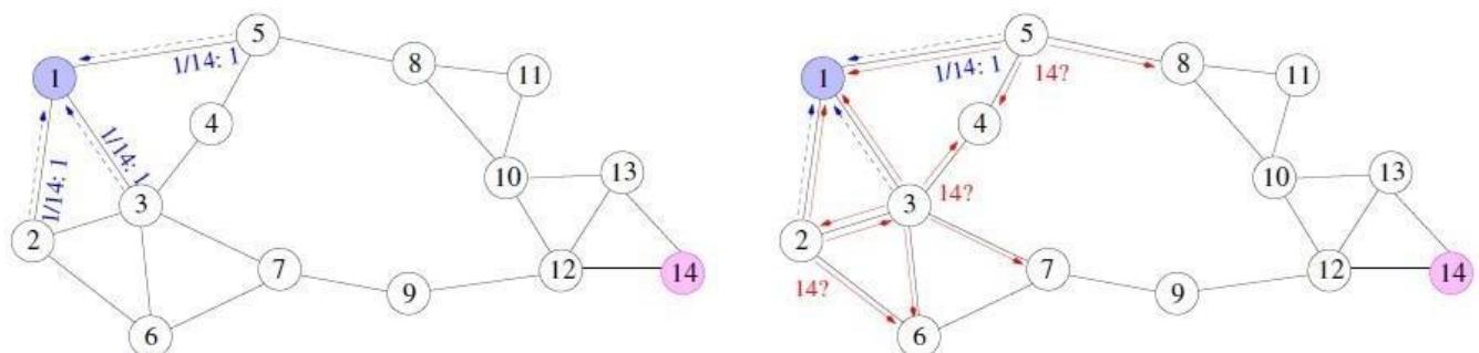
The route request is flooded through the network. Destination managed sequence number, ID prevent looping. Also, flooding is expensive and creates broadcast collision problem.
