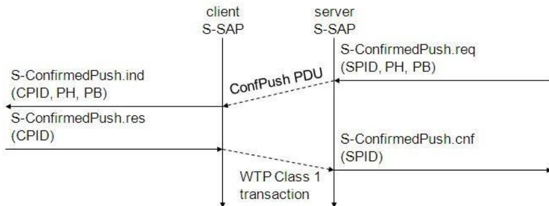
Here the server has to determine the push using a **server push identifier (SPID)**. This helps to distinguish between different pending pushes. The reliable WTP class 1 transaction service is now used to transfer the **confpush PDU** to the client. On the client's side a **client push identifier (CPID)** is used to distinguish between different pending pushes.
