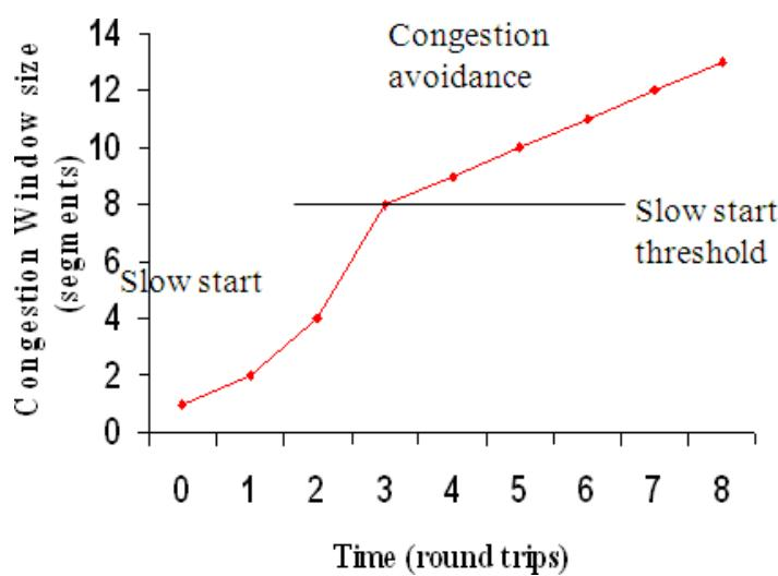
But doubling the congestion window is too dangerous. The exponential growth stops at the **congestion threshold**. As soon as the congestion window reaches the congestion threshold, further increase of the transmission rate is only linear by adding 1 to the congestion window each time the acknowledgements come back.
