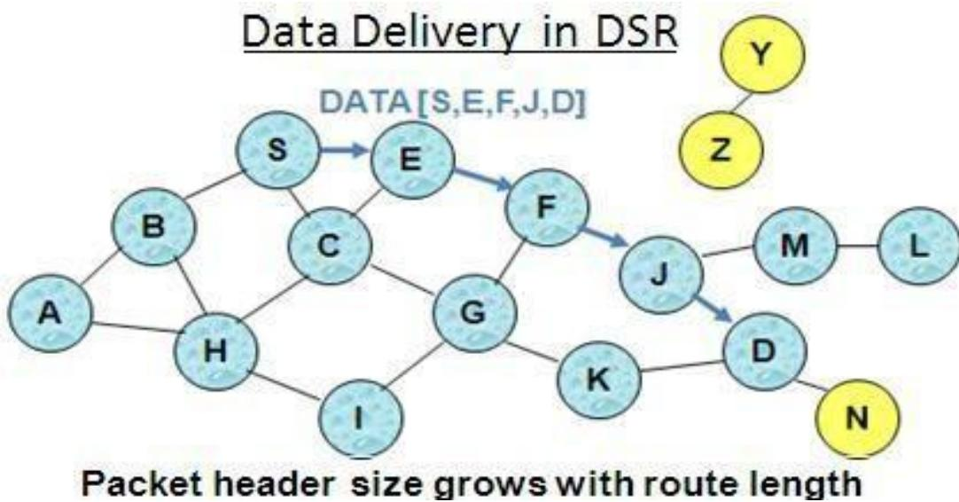
J sends a route error to S along route J-F-E-S when its attempt to forward the data packet S (with route SEFJD) on J-D fails. Nodes hearing RERR update their route cache to remove link J-D
