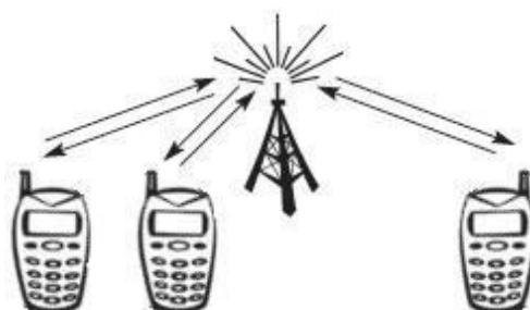
After the busy tone stops, accessing the uplink is not coordinated any further. The base station acknowledges successful transmissions; a mobile station detects a collision only via the missing positive acknowledgement. In case of collisions, additional back-off and retransmission mechanisms are implemented.
