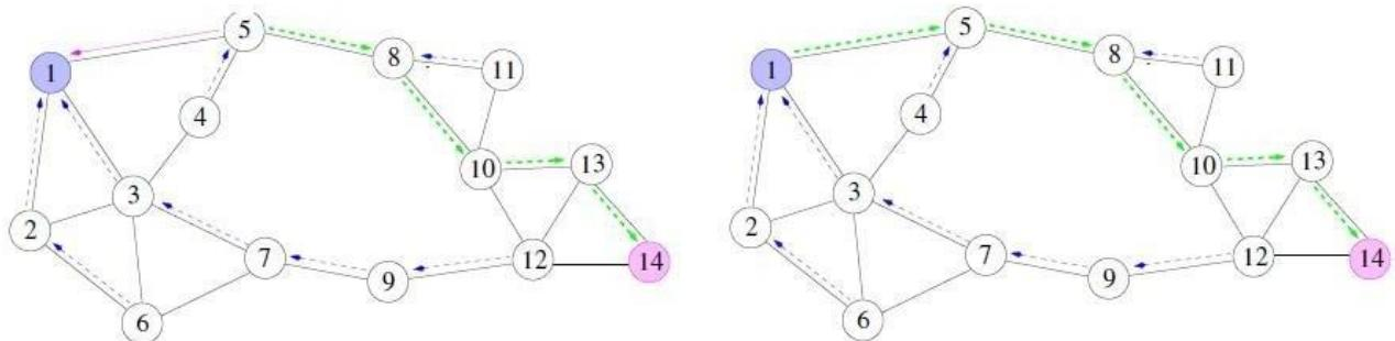
Suppose there has been a failure in one of the links. The node sends a return error message to the source with incrementing the sequence number.
