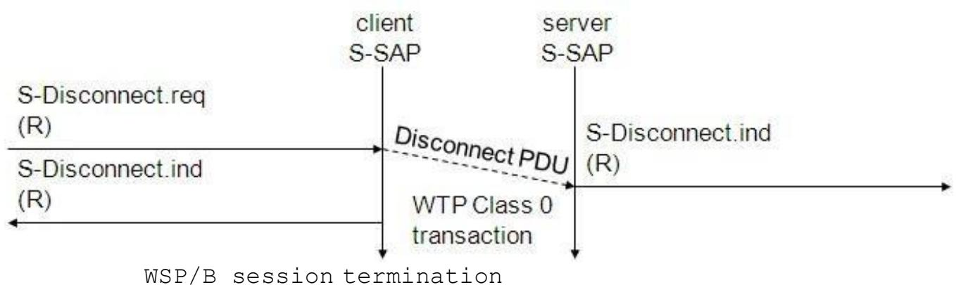
This primitive aborts all current method or push transactions used to transfer data. Disconnection is indicated on both sides using **S-Disconnect.ind**. The **reason R** for disconnection can be, e.g., network error, protocol error, peer request, congestion, and maximum SDU size exceeded.
