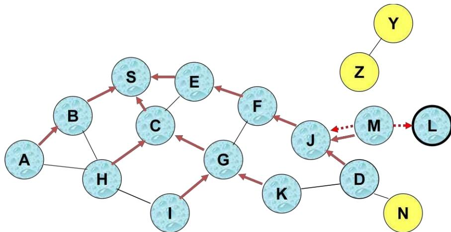
Node D **does not forward RREQ**, because node D is the intended target of the RREQ
