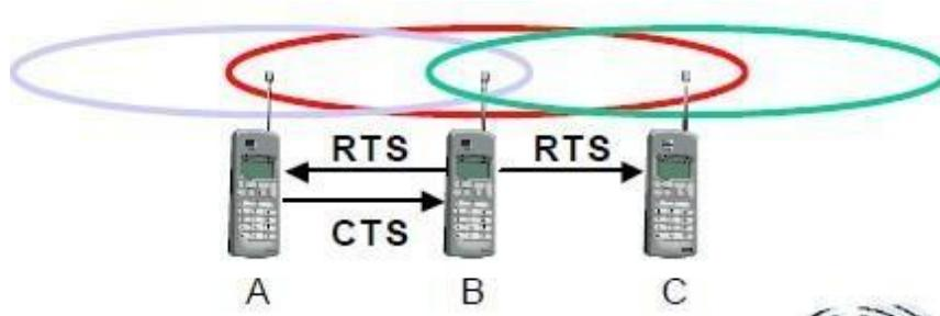
With MACA, B has to transmit an RTS first containing the name of the receiver (A) and the sender (B). C does not react to this message as it is not the receiver, but A acknowledges using a CTS which identifies B as the sender and A as the receiver of the following data transmission. C does not receive this CTS and concludes that A is outside the detection range. C can start its transmission
