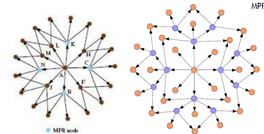
The multipoint relays of each node, (MPR), is the minimal set of 1-hop nodes that covers all 2- hop points.
