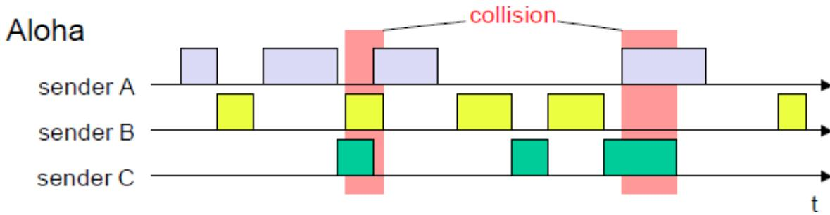
This is a random access scheme, without a central arbiter controlling access and without coordination among the stations. If two or more stations access the medium at the same time, a **collision** occurs and the transmitted data is destroyed. Resolving this problem is left to higher layers (e.g., retransmission of data). The simple Aloha works fine for a light load and does not require any complicated access mechanisms.
