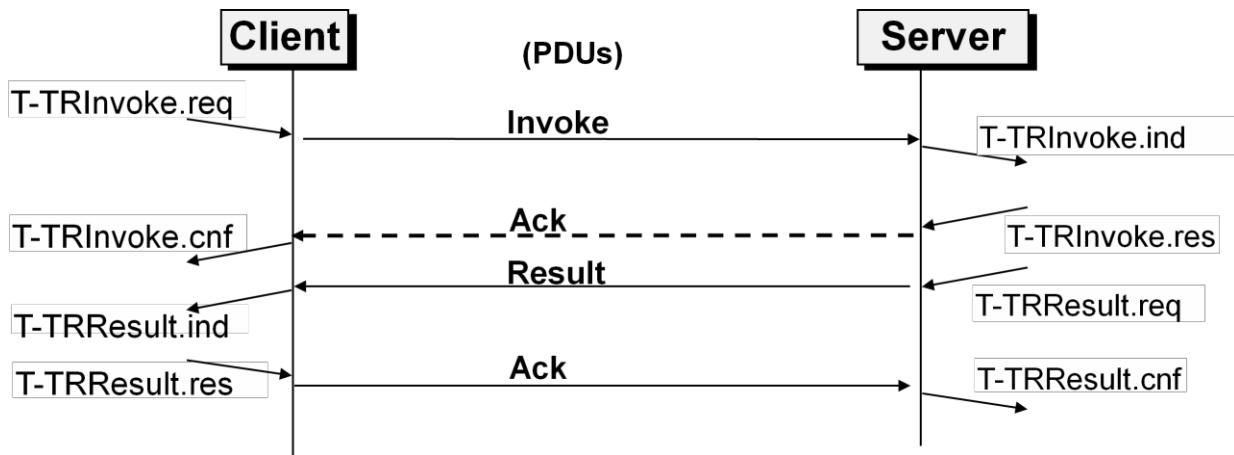
The PDUs exchanged between two WTP entities for normal transactions are the **invoke PDU**, **ack PDU**, and **result PDU**. A special feature of WTP is its ability to provide a **user acknowledgement** or, alternatively, an **automatic acknowledgement** by the WTP entity.
