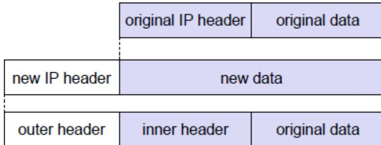
**Encapsulation** is the mechanism of taking a packet consisting of packet header and data and putting it into the data part of a new packet. The reverse operation, taking a packet out of the data part of another packet, is called **decapsulation**. Encapsulation and decapsulation are the operations typically performed when a packet is transferred from a higher protocol layer to a lower layer or from a lower to a higher layer respectively.
