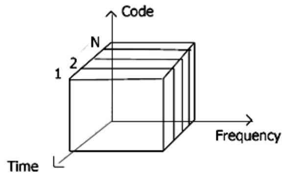
Listening to different frequencies at the same time is quite difficult, but listening to many channels separated in time at the same frequency is simple. Fixed schemes do not need identification, but are not as flexible considering varying bandwidth requirements.
