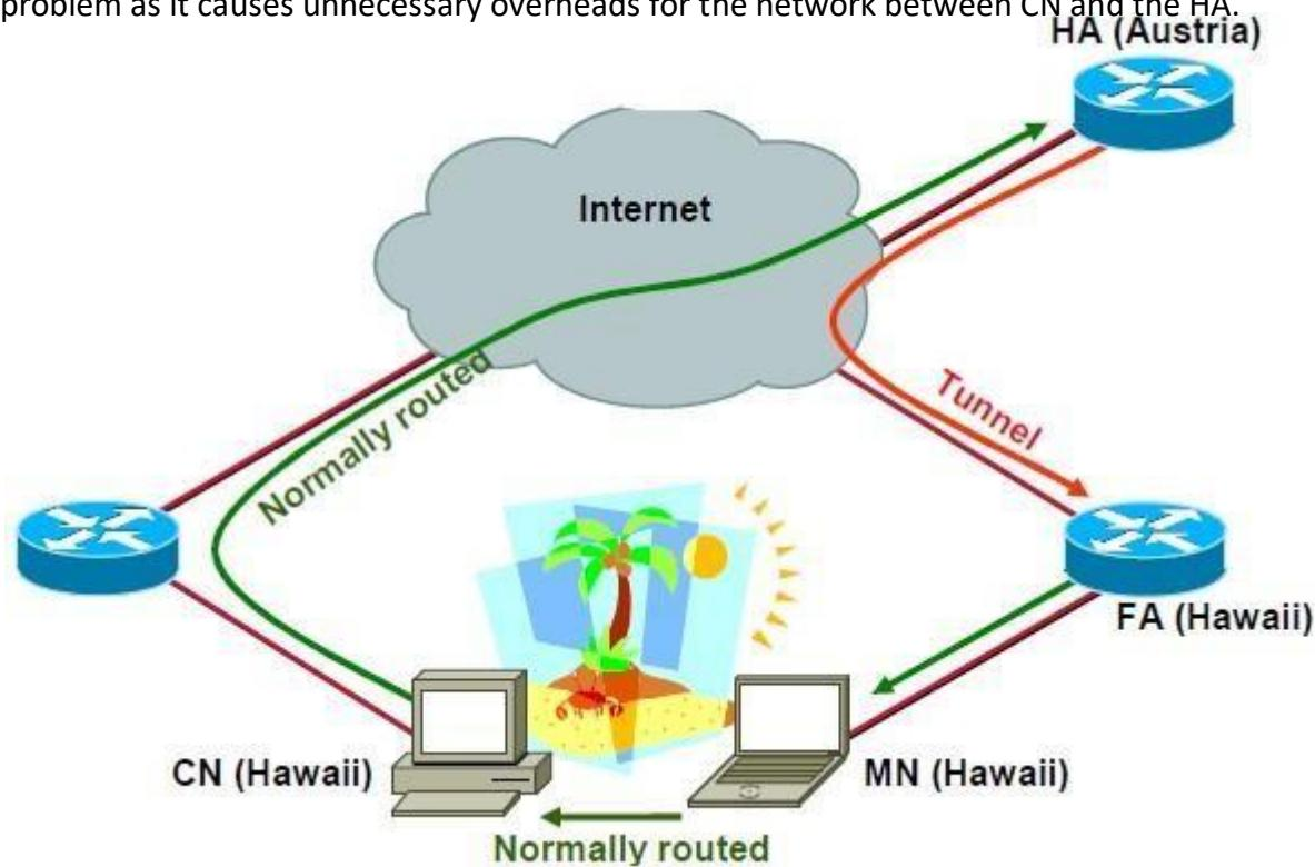
A solution to this problem is to inform the CN of the current location of the MN. The CN can learn the location by caching it in a binding cache, which is a part of the routing table for the CN. HA informs the CN of the location. It needs four additional messages:
