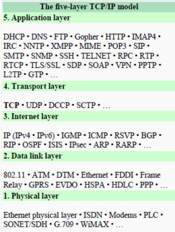
TCP supports many of the Internet's most popular application protocols and resulting applications, including the World Wide Web, e-mail, File Transfer Protocol and Secure Shell. In the Internet protocol suite, TCP is the intermediate layer between the Internet layer and application layer.
