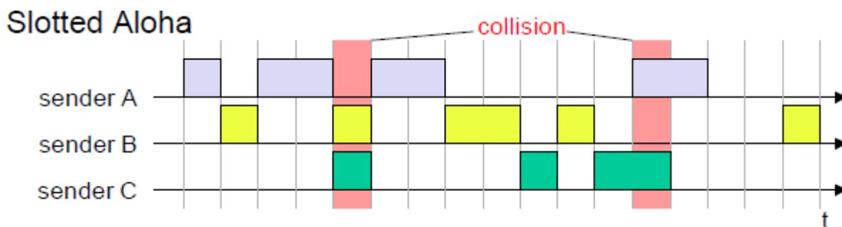
The introduction of slots raises the throughput from 18 per cent to 36 per cent, i.e., slotting doubles the throughput. Both basic Aloha principles occur in many systems that implement distributed access to a medium. Aloha systems work perfectly well under a light load, but they cannot give any hard transmission guarantees, such as maximum delay before accessing the medium or minimum throughput.
