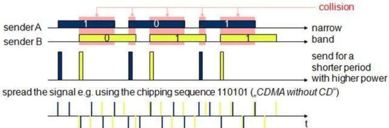
The main problem in using this approach is finding good chipping sequences. The maximum throughput is about 18 per cent, which is very similar to Aloha, but the approach benefits from the advantages of spread spectrum techniques: robustness against narrowband interference and simple coexistence with other systems in the same frequency bands.
