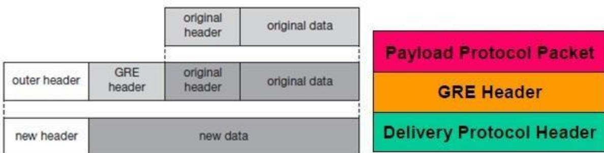
The packet of one protocol suite with the original packet header and data is taken and a new GRE header is prepended. Together this forms the new data part of the new packet. Finally, the header of the second protocol suite is put in front. The following figure shows the fields of a packet inside the tunnel between HA and COA using GRE as an encapsulation scheme according to RFC 1701. The outer header is the standard IP header with HA as
