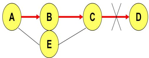
Assume that A does not know about failure of link C-D because RERR sent by C is lost.
