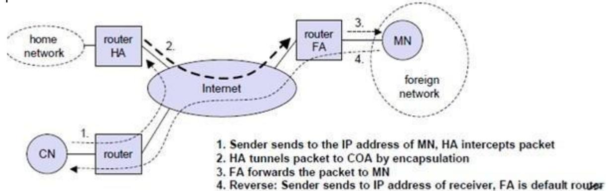
CN sends an IP packet with MN as a destination address and CN as a source address. The internet, not having information on the current location of MN, routes the packet to the router responsible for the home network of MN. This is done using the standard routing
