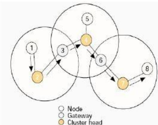
The cluster structure leads to a higher performance of the routing protocol as compared to other protocols because it provides gateway switch-type traffic redirections and clusters provide an effective membership of nodes for connectivity.
