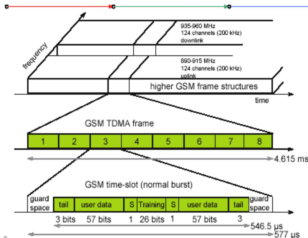
GSM TDMA Frame, Slots and Bursts
