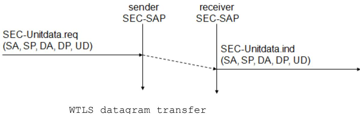
After setting up a secure connection between two peers, user data can be exchanged. This is done using the simple **SEC-Unitdata** primitive as shown in above figure. SEC-Unitdata has exactly the same function as T-DUnitdata on the WDP layer, namely it transfers a datagram between a sender and a receiver. This data transfer is still unreliable, but is now secure. This shows that WTLS can be easily plugged into the protocol stack on top of WDP.
