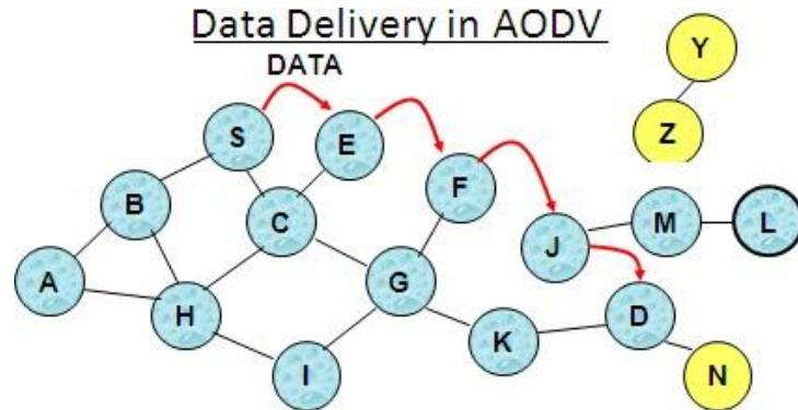
Routing table entries used to forward data packet.
