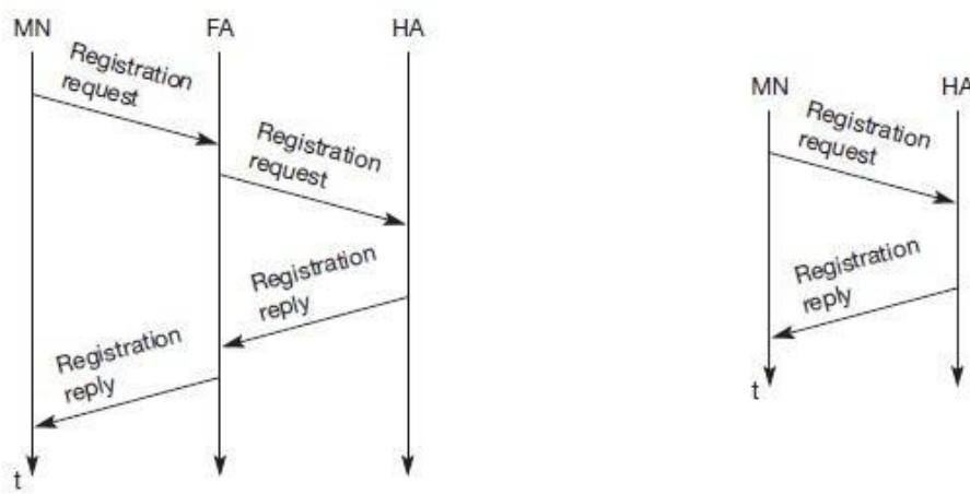
Registration of a mobile node via the FA or directly with the HA
