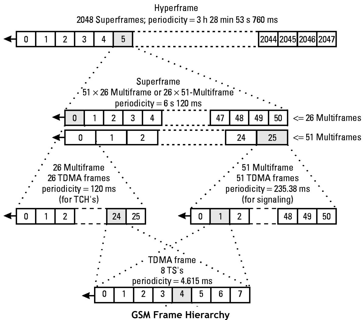
There are two different types of logical channel within the GSM system: Traffic channels (TCHs), Control channels (CCHs).
