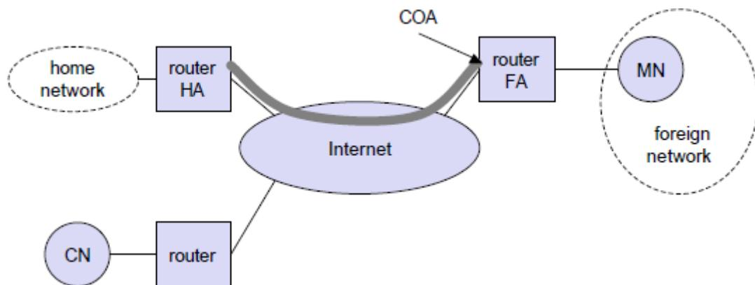
A CN is connected via a router to the internet, as are the home network and the foreign network. The HA is implemented on the router connecting the home network with the internet, an FA is implemented on the router to the foreign network. The MN is currently in the foreign network. The tunnel for packets toward the MN starts at the HA and ends at the FA, for the FA has the COA in the above example.
