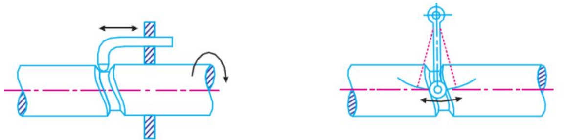
(a) Cylindrical cam with reciprocating follower.
